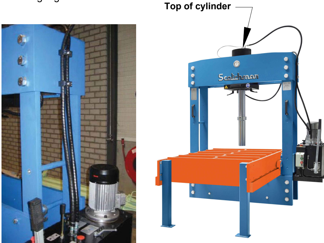
Fig. 6 Keep hoses straight - no sharp bends
